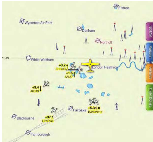
Figure 4: uAvionix receivers connect to a number of existing airspace awareness apps using a Wi-Fi hotspot connection and GDL90 protocol.
