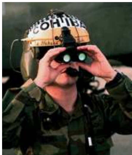
Figure 7 US pilot adjusts his Night Vision Device before flying. ©DoD Public Domain
