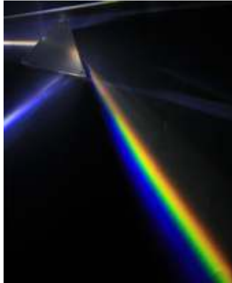
Figure 9. White light analysis by dispersion using a prism. Public Domain
